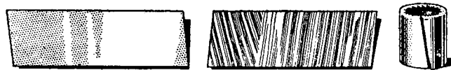
FIG. 9.—The iron lining for a “ Gas-Tight ” case : plain, varnished and rolled and shaped.
